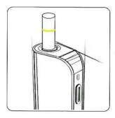
a) Preparation: Load the iBuddystick Holder into the heating device, then insert a stick into the Holder.
