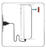
j).Charging: Insert the USB charging cable under Standby Mode, the red light turns on and the device enters Charging Mode. When charge is completed, the red light turns off and the device enters Standby Mode.
