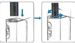
Rotate the brush to clean the heating pin
