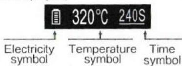
b. Start-up preheating interface(Press the power button for 3 seconds, then the device vibrates, heating& characters flickering, After 10 seconds, it reaches the set temperature and enters the smoking status)
