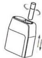
1.3 Protective cover of Heating rod (The cartridge holder is made of special PEEK material, Forbid opening the protective cover when heating,you can clean the heating rod after cooling and pull up protective cover.
