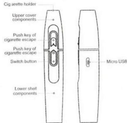
Fig.1 Structural Configuration
